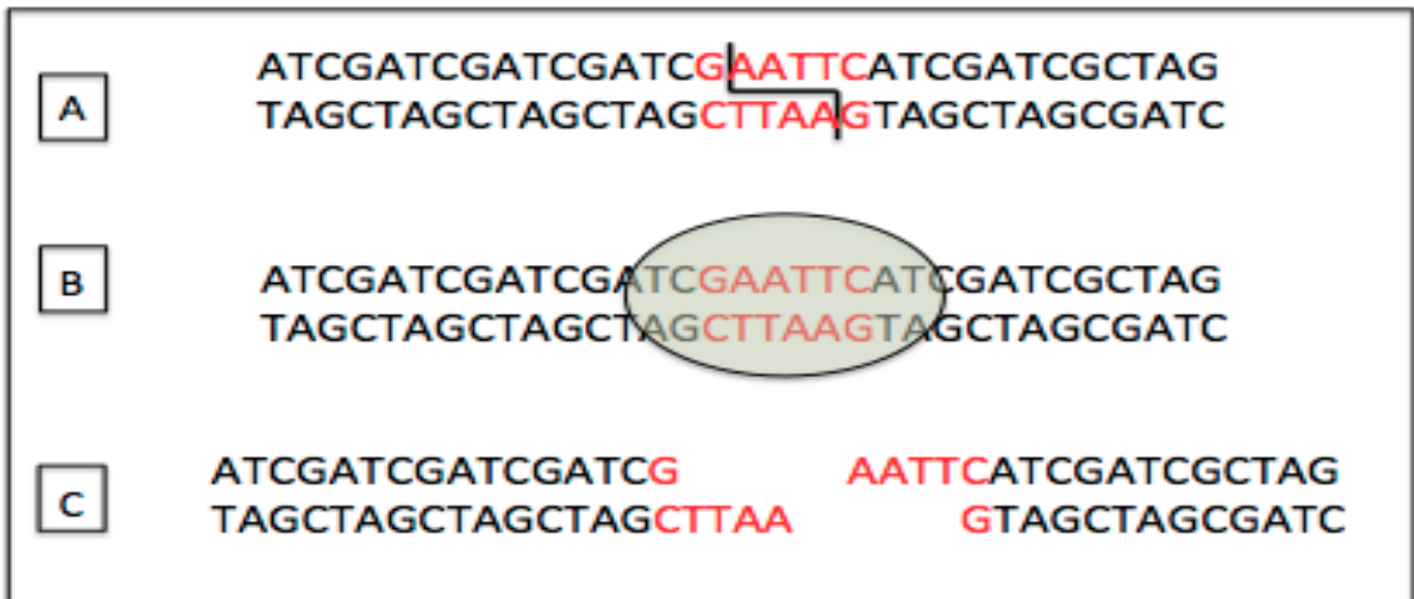
Figure 11: Principle of restriction enzymes cutting site_
